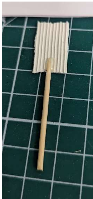
Fig 42. Section of wafer mounted on cocktail stick
