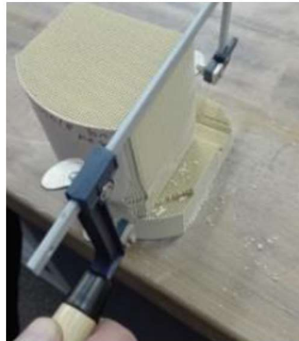
Fig 13. Cutting wafers with piercing saw and wafer sealed in holder
