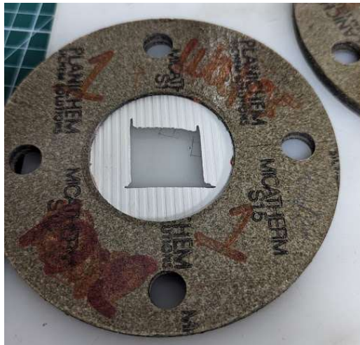
Fig 41. Section of wafer removed from sample from experiments.
