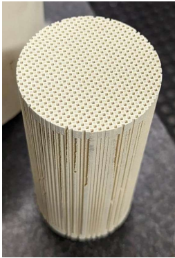
Fig 11. Core cut from full size filter.
