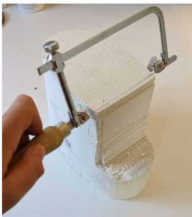
Fig 17. Cutting wafer from full size filter.
