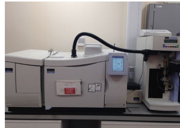
Thermo-gravimetric Analyser (TGA) Gas Chromatograph (GC) Mass Spectrometer (MS)
